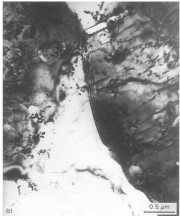
Figure 7 Transmission electron micrographs of the (a) as-received and (b) pre-strained specimens, deformed at temperature of 517^\circ\text{C} and strain rate of 2 \times 10^{-4} \text{ s}^{-1} to a true strain of 1.4 (elongation = 305%).
